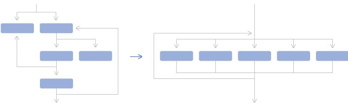
Flattening the control flow, a common code obfuscation technique.
